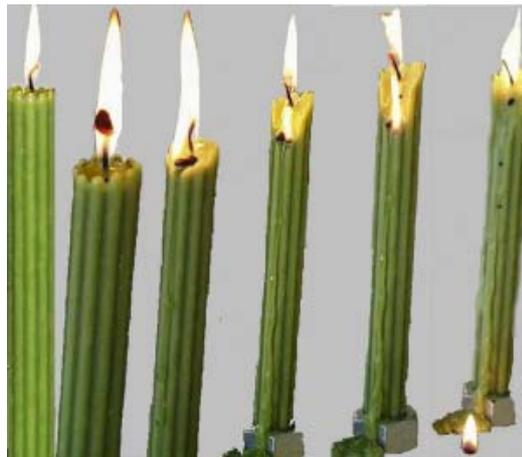
**Figure 18: Formation of Second Wicks Caused by Debris Resulting from Mushrooming**
