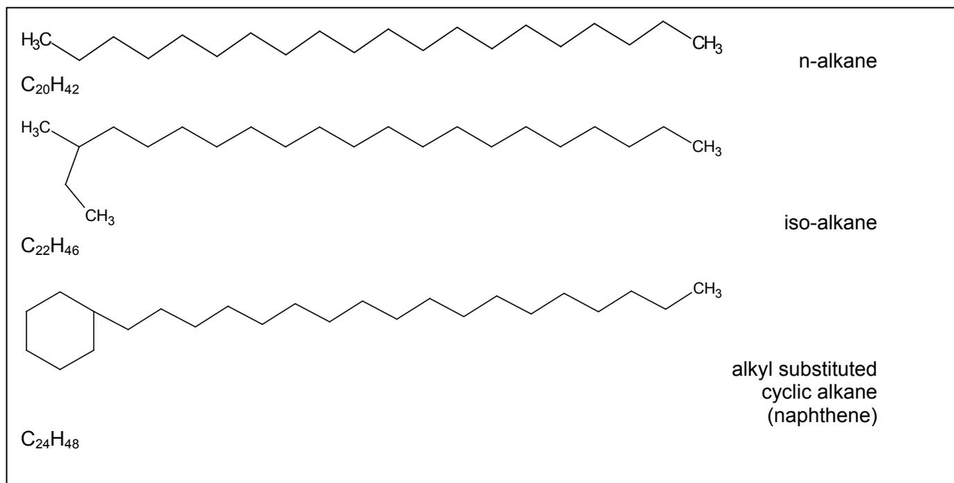
Figure 5: Paraffin Wax; Examples of Chemical Structures
