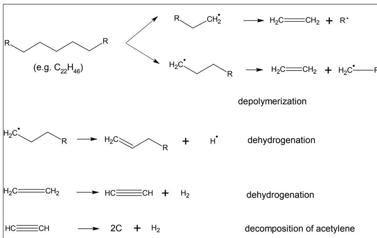
Figure 15: Mechanism of Chain Degradation Within the Flame
