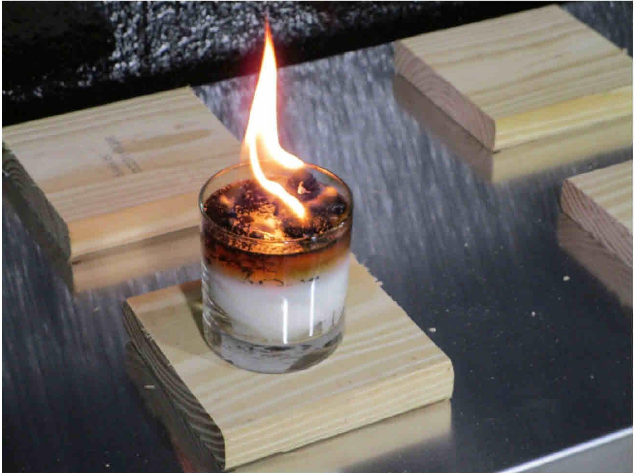
Figure 6: Sample 1 Company candle. Within 50 minutes of lighting, candle experienced flashover where entire surface is on fire.
