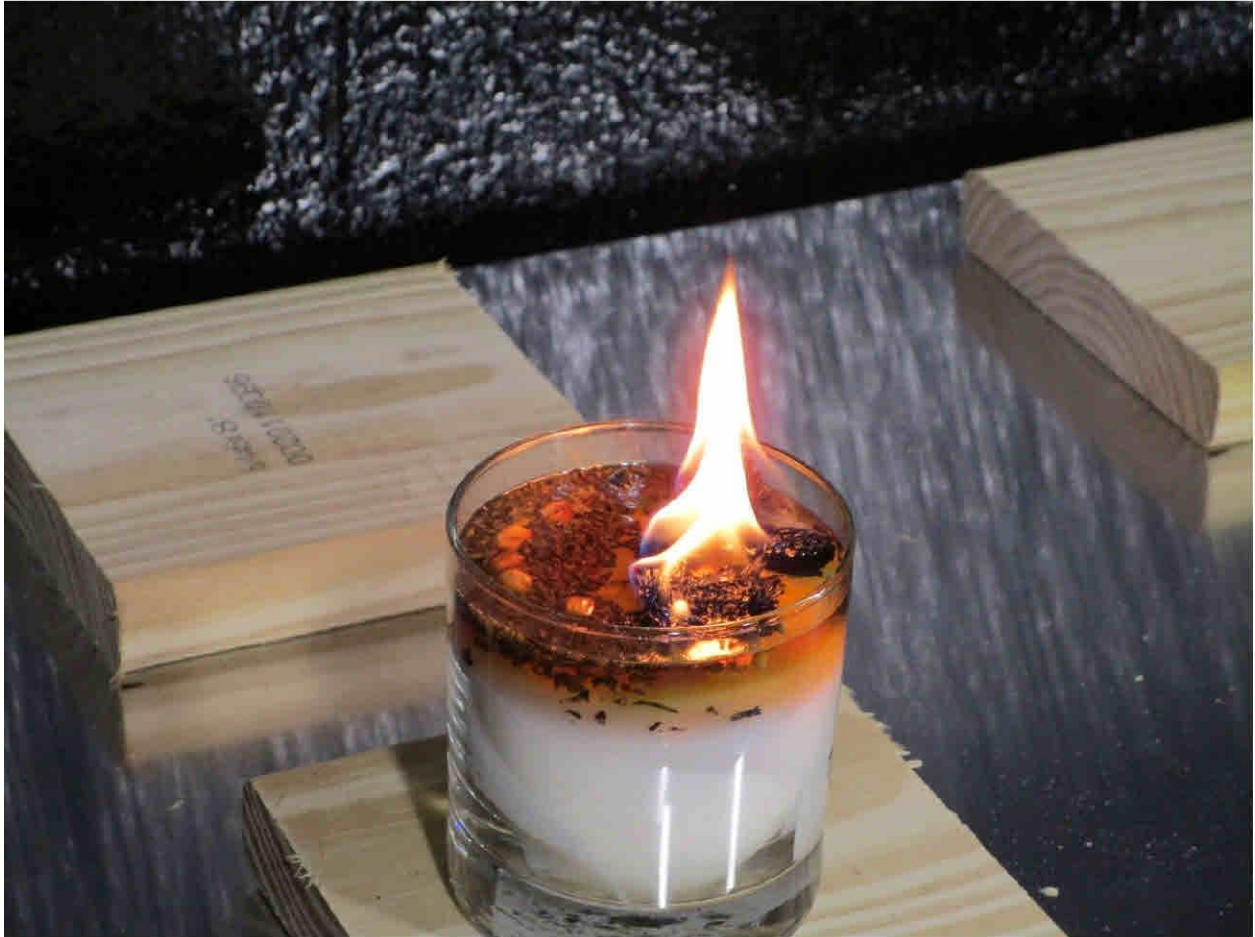
Figure 5: Sample 1 Company candle with secondary ignition progressing. Wax pool is becoming deep.
