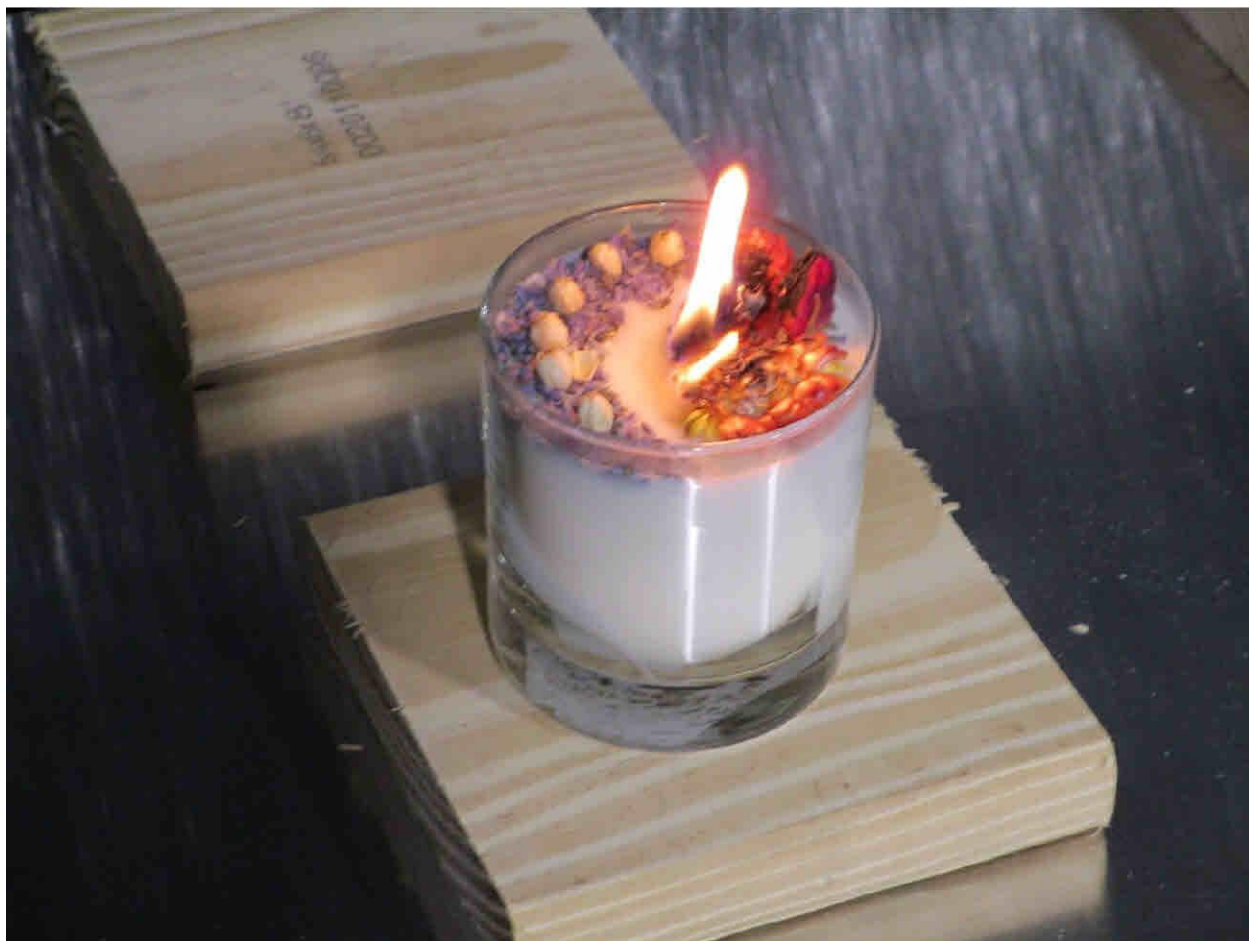
Figure 4: Sample 1 Company candle shortly after lighting. Dried flower has ignited and is supporting combustion.
