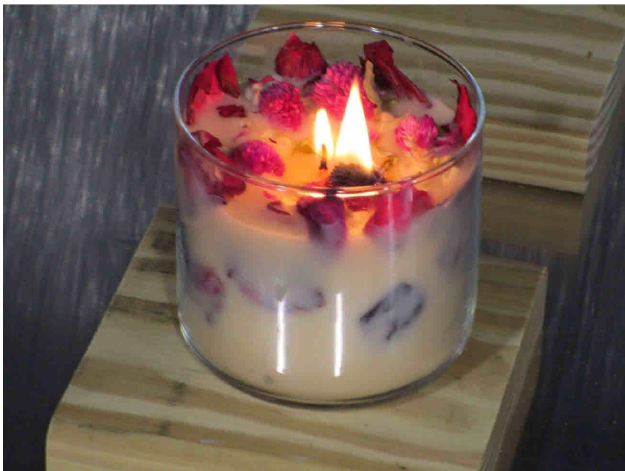
Figure 7: Sample 3 Company candle, with secondary ignition of botanicals, during first four-hour burn cycle.
