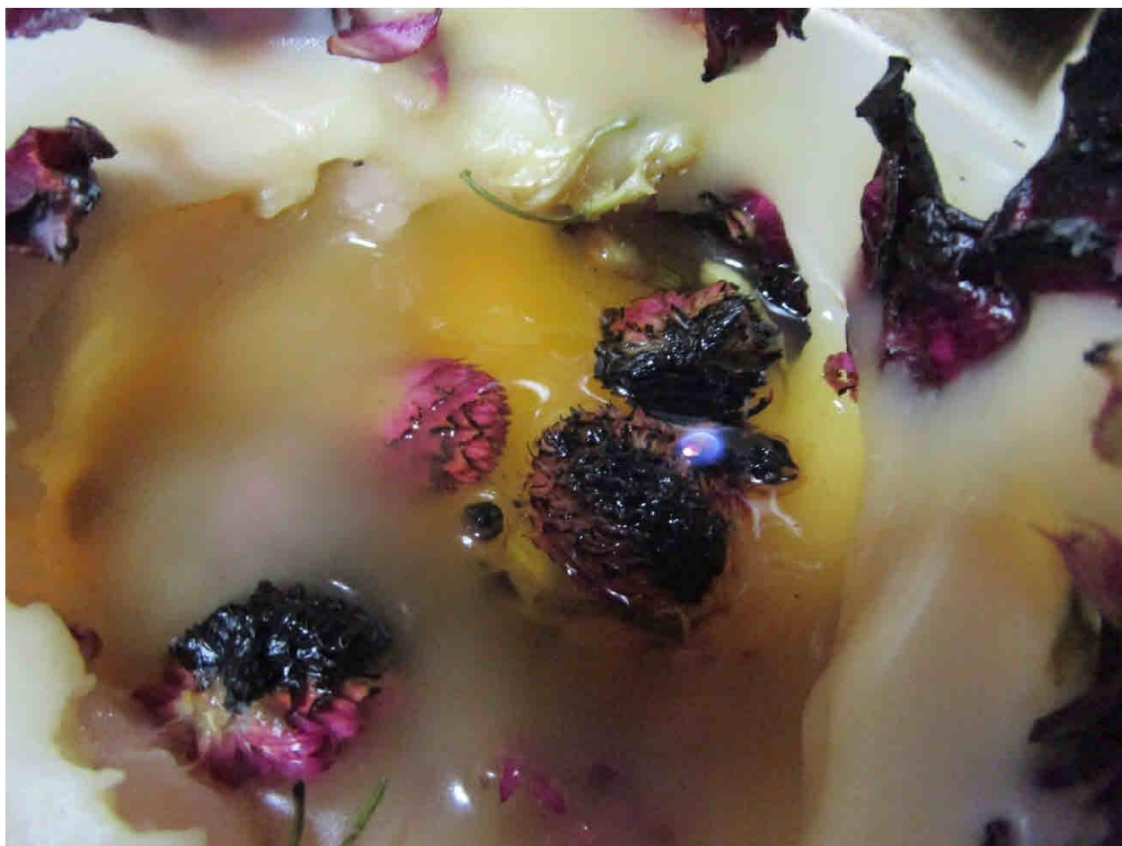
Figure 8: Thirty minutes after lighting Sample 3 Company candle last time. Only botanicals remain lit and wax pool drowns out flame on wick.
